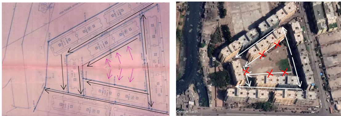
Figure 3.11 Image highlighting the currents status of SWD channels. Where cross marked drain channels along the edges of maidan has been completely closed by locals.
